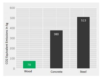
This chart shows how many kilograms of CO2 are generated to create a beam 7.3m (24') long, supporting 14.4kN/m (1,060 lbs/ft), in three materials. Numbers do not include CO2 sequestered in materials.
